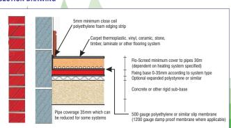
**SIGNIFICANT REDUCTIONS IN THICKNESS** · In most cases 35mm of Flo-screed will replace 75mm of conventional material.
